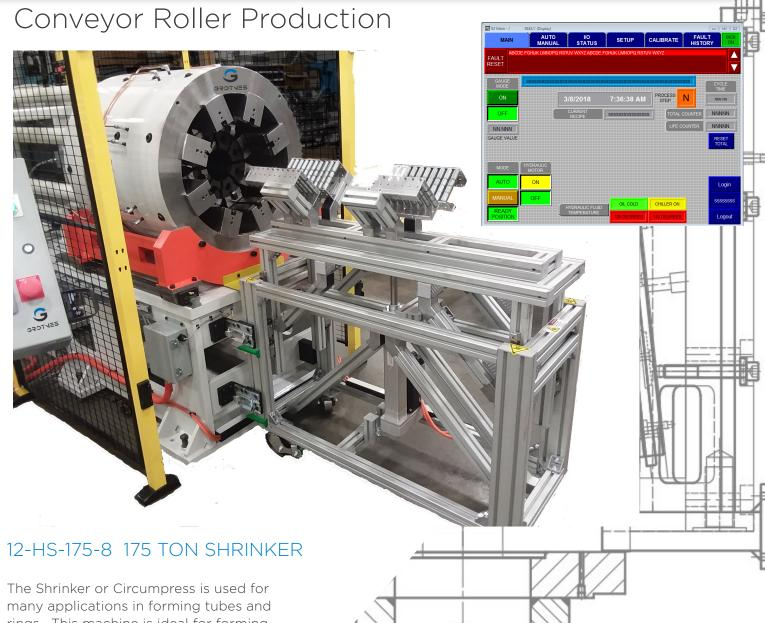
rings. This machine is ideal for forming tapered rollers for conveyors. The tooling is easily changed for different diameters and/or taper angles.
